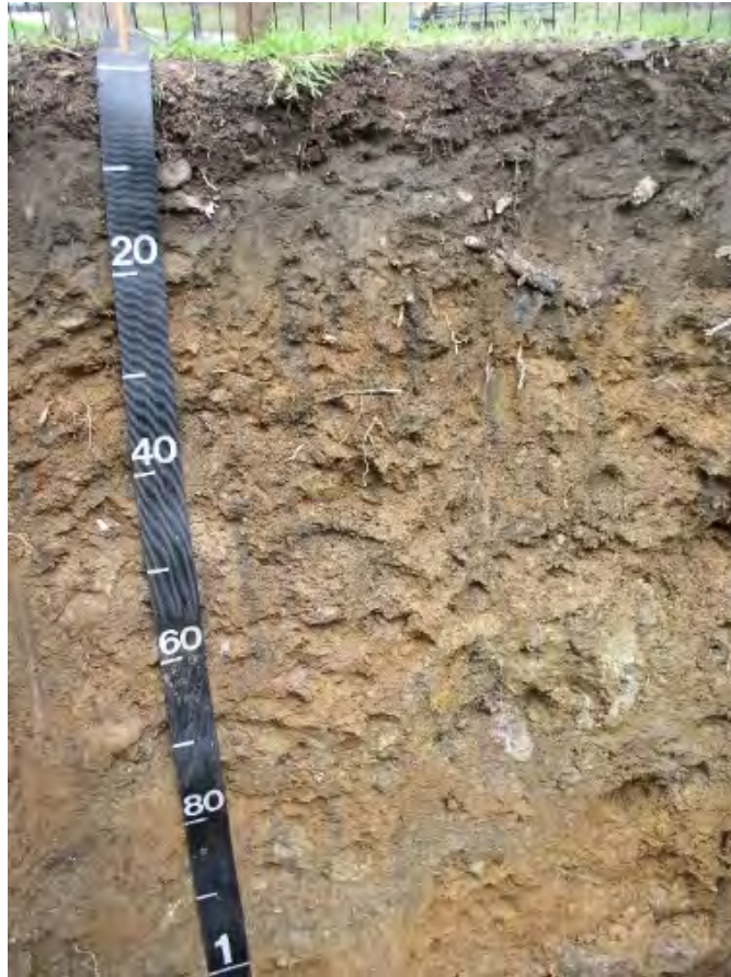
Photo 19. Soil profile, Spodic HAHT material class. North Meadow soil series, Central Park, New York, NY, United States of America, containing 364.91 t SOC/ha
